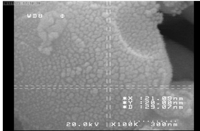
Figure 1a. SEM photo of produced zinc oxide nano particles.
