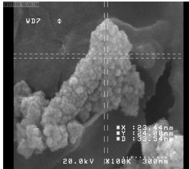
Figure 1b. SEM photo of produced zinc oxide nano particles.
