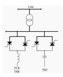
Fig. 2. Static Var Compensator (SVC)
