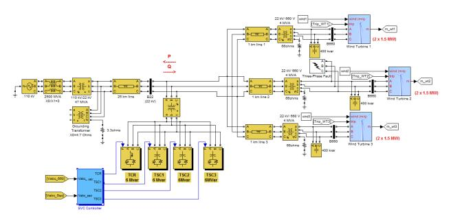
Fig. 4. Matlab-Simulink simulation of a wind power station connected to the grid
