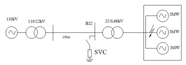
Fig. 3. Model of wind power station connected with national grid
