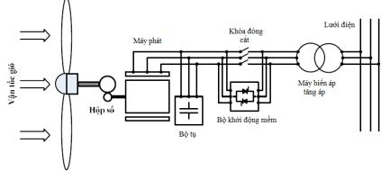
Fig. 1. The connection diagram of wind power station and national grid
