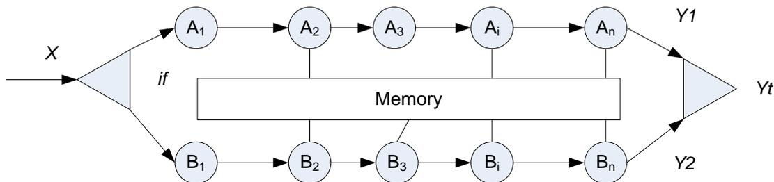
Fig. 3. Logical sequence in parallel information processing
